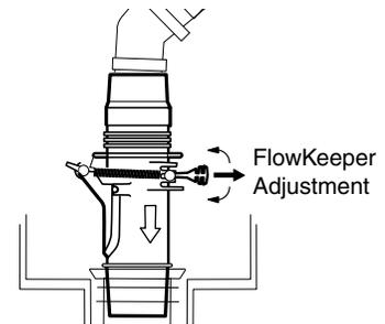
If the pool has more than one skimmer, connect the hose to the one closest to the pump.
